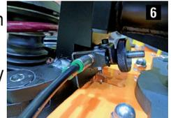
When the operations are complete, de-risk the shock absorber removal tool by disconnecting the air supply.
